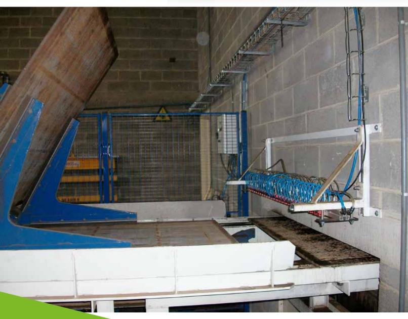
Spraying ramp for a concrete blocks production line (Wooden Boards | Steel Boards | Composite Boards)
